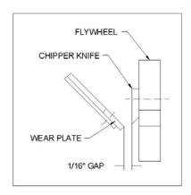
NOTE: Proper gap setting is critical to the proper operation of your machine.
